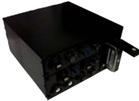
ARS Control and Processing Unit
